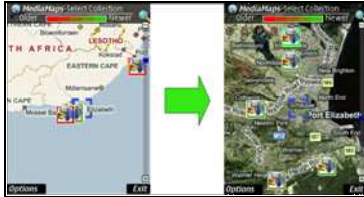
Fig. 2. Visualization adaptation in MediaMaps, before adaptation (left) and after adaptation (right)
