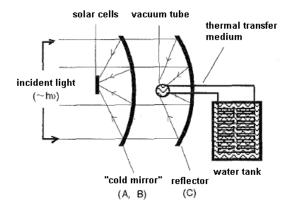
Fig. 1. A schematic structure of a concentrating PV/T collector [6].
