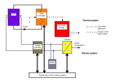
Fig. 3. Block diagram of PV/T system.
