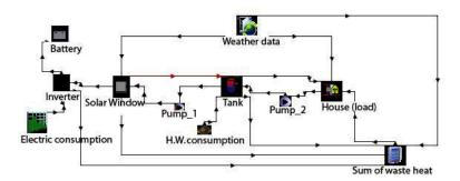
Fig. 4. Block diagram of a PV/T TRNSYS model [21].
