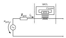
Fig. 5. Inductive superconducting fault current limiter electrical diagram.
