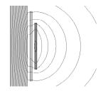
**Fig. 6.** Axisymmetric representation of an inductive SFCL in normal operation. Primary's flux is shielded from iron core by HTS induced currents.
