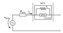
Fig. 2. Resistive superconducting fault current limiter electrical diagram.
