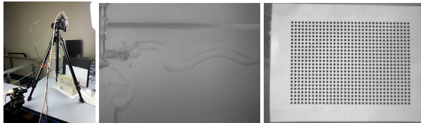
Fig. 2: (left) Experimental setup, showing the top and side camera, observing the silicon vascular phantom; (middle) image of the phantom by the top camera; (right) calibration pattern used to compute the equation of the refractive plane (inter-bullet distance=2 mm)
