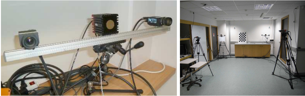
Figure 1: A single ToF+2RGB system (left), comprising a time-of-flight camera in the centre, plus a pair of ordinary colour cameras. This paper addresses the problem of simultaneously cross-calibrating many such systems (right), as a foundation for scene understanding
