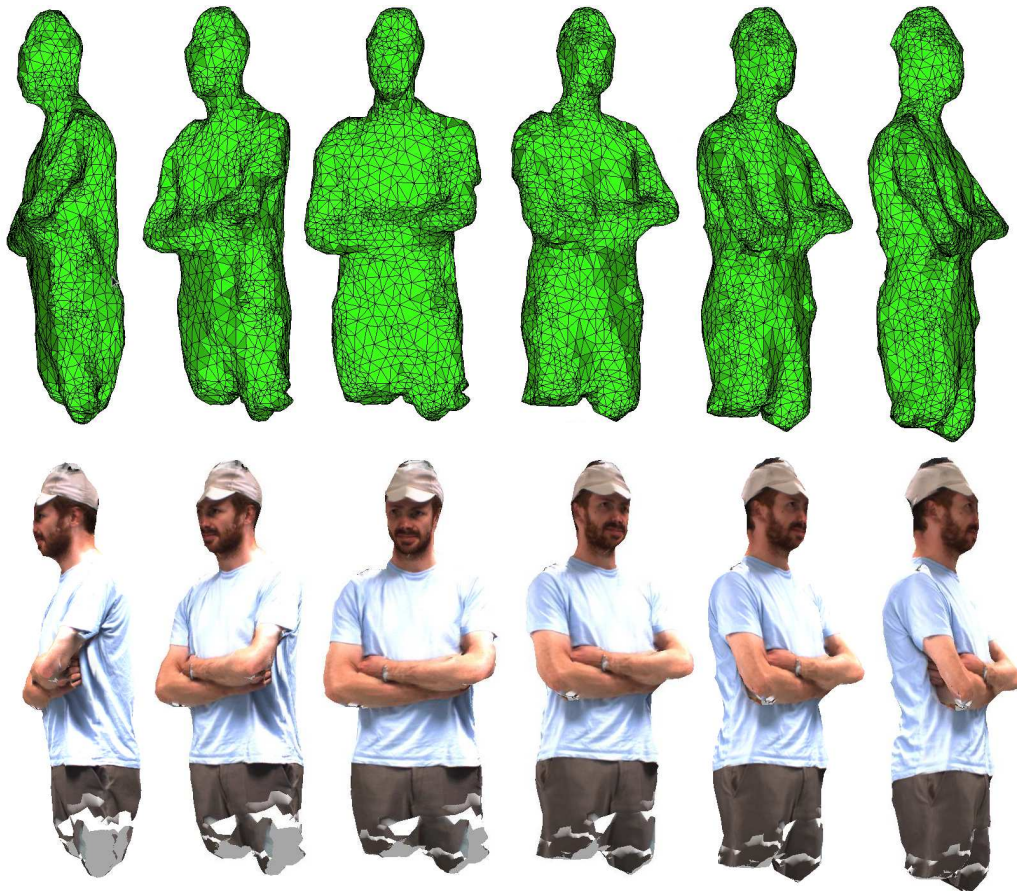
Figure 11: Examples of a segmented 360° reconstruction, after Poisson meshing, with and without RGB texture.
