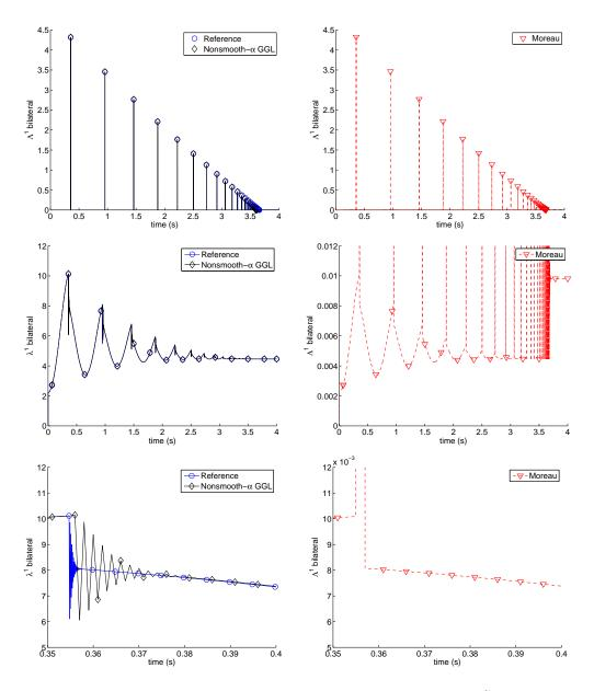
Figure 13: Bouncing pendulum: bilateral multipliers (first column:  $\Lambda^1$ ,  $\tilde{\lambda}^1$  and zoom on  $\tilde{\lambda}^1$ ; second column:  $\Lambda^1$ , zoom 1 on  $\Lambda^1$  and zoom 2 on  $\Lambda^1$ ).
