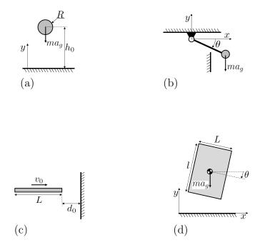
Figure 1: Examples: (a) bouncing ball; (b) rigid pendulum; (c) elastic bar; (d) rocking block.
