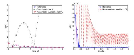
Figure 2: Bouncing ball: gap distance and zoom.
