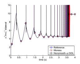
Figure 15: Bouncing pendulum: bilateral reaction force  $\Lambda^1/h + \tilde{\lambda}^1$ .
