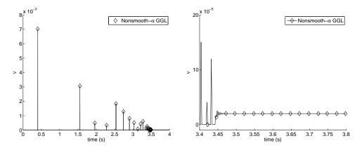
Figure 7: Bouncing ball: Lagrange multiplier  $\nu$  and zoom.
