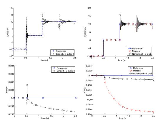
Figure 18: Bar impact: velocity and energy.
