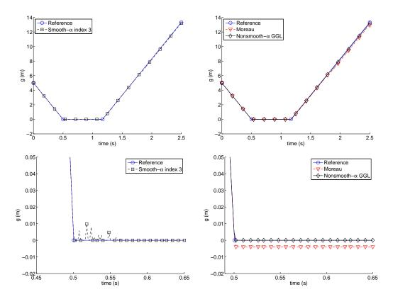
Figure 17: Bar impact: gap distance and zoom.
