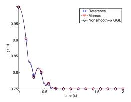
Figure 20: Rocking block: vertical position.
