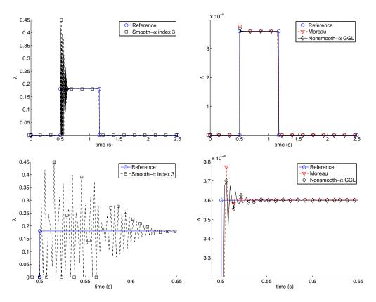
Figure 19: Bar impact: unilateral Lagrange multiplier  $\Lambda$  and zoom.
