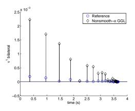
Figure 16: Bouncing pendulum: bilateral multiplier  $\nu^1.$
