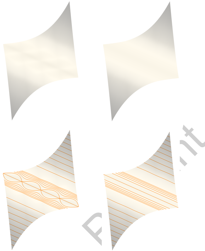
Fig. 9 Interpolation of a grid sampled from an analytical function. The left part shows the result when the exact partial derivatives of the function are used for the interpolant. The isolines on the bottom left clearly indicate critical points. In the right part these critical points are removed by modifying the partial derivatives with our Algorithm 1 (Section 3.4).
