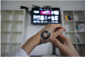
Figure 1: Prototype used for remote TV control
