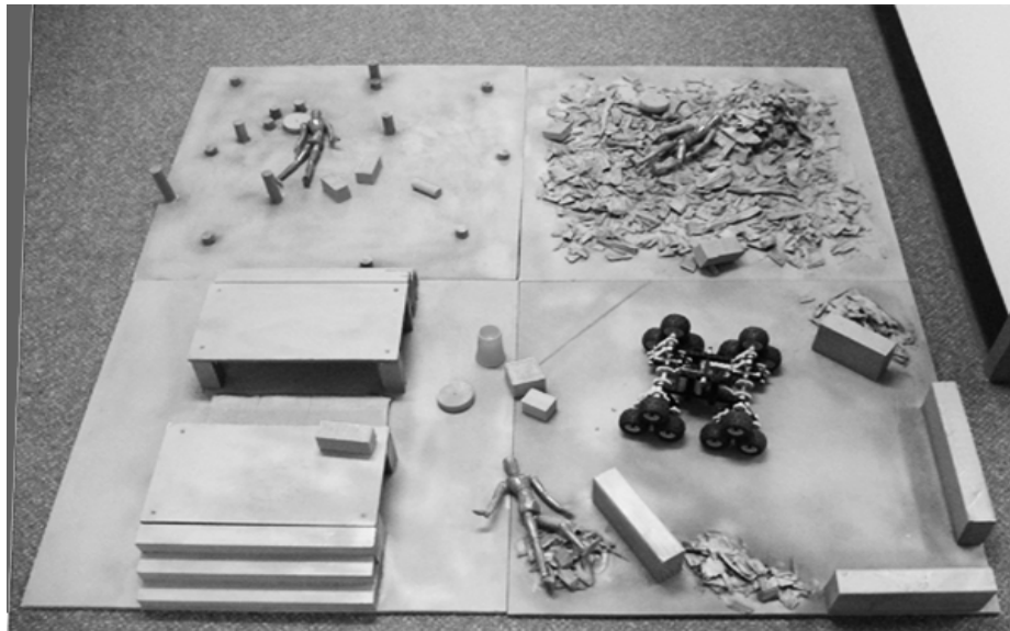
Fig. 3. 3-dimensional search and rescue robot arena. Four platform tiles arranged in a geomorphic configuration. The arena is populated with scaled-down effigies of victims, debris and moveable objects.
