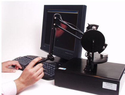
Fig. 13. The 6 DOF Phantom haptic device
