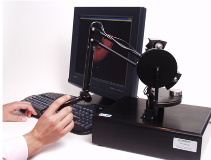
Fig. 13. The 6 DOF Phantom haptic device
