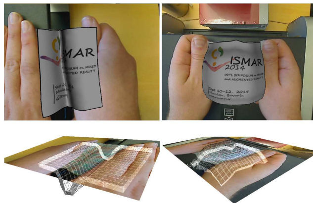
Figure 1: Three-dimensional reconstruction and augmentation of elastic objects from a single view under several elongations. Our approach is able to handle extensibility of the material when undergoing elongation. In (top) the camera view of the re-textured elastic object and in (bottom) the recovered 3D shape form showed from a different view.
