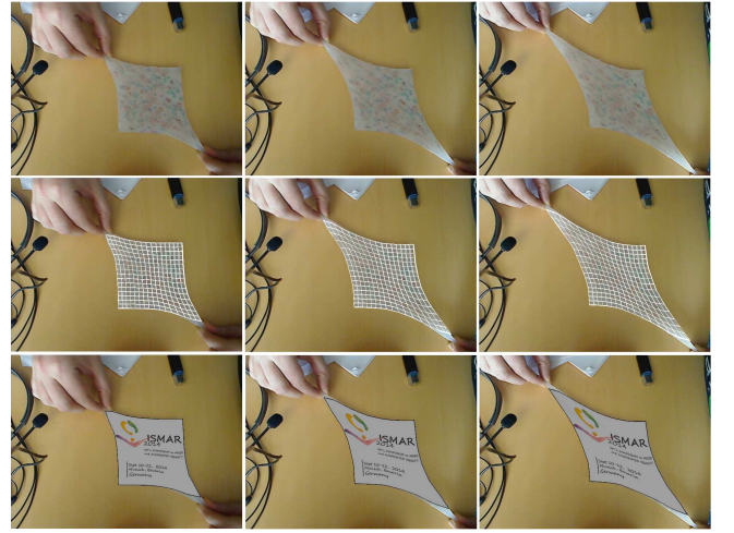
Figure 5: Selected frames during a 2D elastic surface augmentation of the silicone-like material when being stretched up to 120%, with (top) input images (middle) registered mesh (bottom) surface retexturing.
