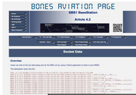
ADS-B Message format and SBS1 specification
