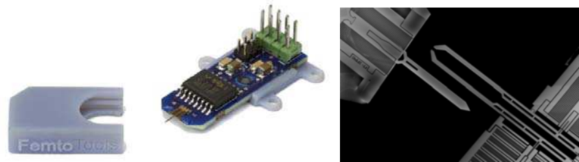
Fig. 5: Force sensor. System overview (left) and close-up view (courtesy of FemtoTools).
