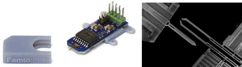
Fig. 5: Force sensor. System overview (left) and close-up view (courtesy of FemtoTools).
