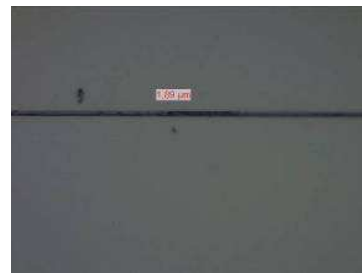
Fig. 8. : Adhesive gap of < 3 μm
