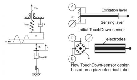
**Fig. 3.** Mechanical model for the TouchDown-sensor, modeled as a spring-mass-damper system. The contact between the object, e.g. CNT, is modeled as a second damper (left). The mechanical setup for both approaches is schematically depicted (right).
