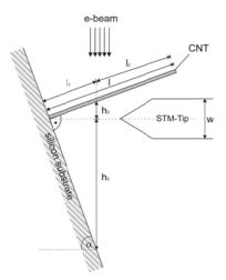
**Fig. 2.** Side view of the scene for the assembly of CNTs. The CNT is grown on a silicon substrate, which is mounted with a tilt angle in the SEM. The CNT is approached by a fine etched metal tip. A possible contact needs to be detected in all three dimensions.
