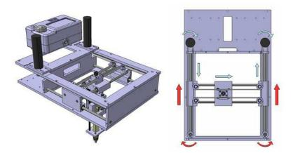
Fig. 3. CAD-model of the H-type structure
