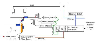
Fig. 8. Control system of the screwing cell
