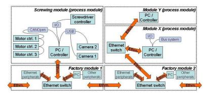
Fig. 7. Control system architecture between the modules
