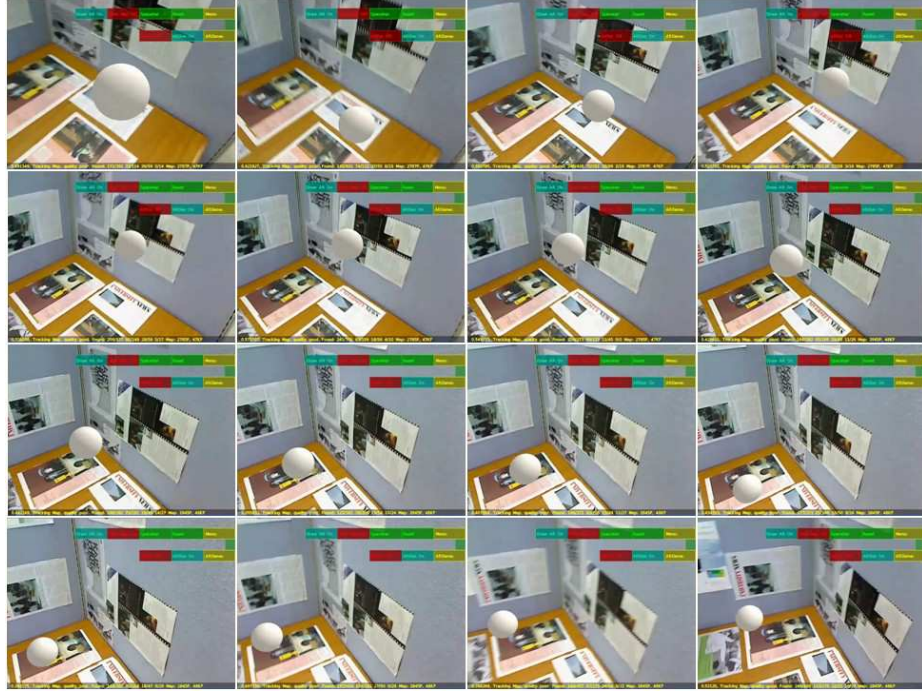
Fig 8. A virtual gravity ball rebounding from real ground and walls
