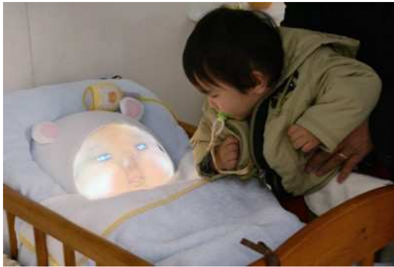
Fig. 1 Physical appearance of baby-type robot “YOTARO”
