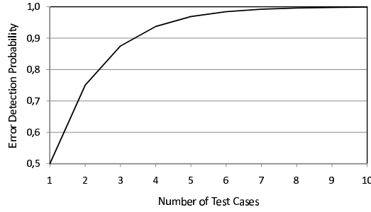
Fig. 2. Error Detection Probability of MC/DC [1]
