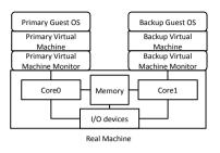
Fig. 1. Overall Architecture of the Proposed System
