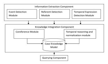
Fig. 1. Overall architecture of the knowledge-based system.
