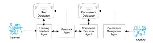
Figure 1. Adaptive WBI architecture and components
