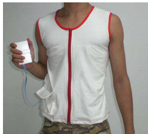
Fig. 7. A prototype of e-Textcare® wearable multi-functional physiological measurement system.
