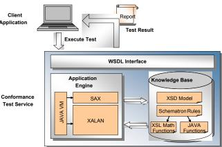
Fig. 3. Architecture for CT system validation [24]
