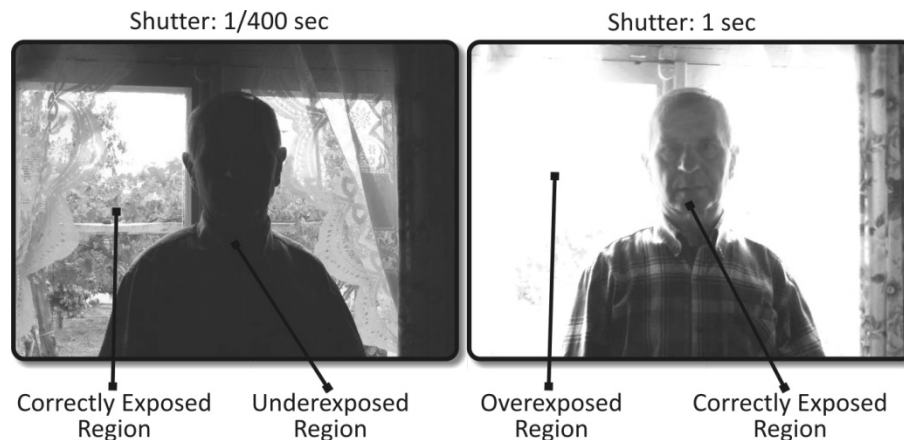
Figure. 1. There is not a single exposure that can adequately capture both the dark and light regions of an HDR scene.
