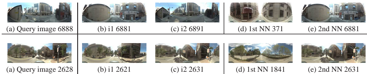
Figure 9. Examples of correct localization on the map with sampling rate \Delta = 5 using the proposed method. (a) Query image. (b-c) The image pair selected by the proposed matching of linear combinations of image descriptors (correct). (d-e) The first two nearest neighbors (1st NN is incorrect). The distance between images (b) and (c) on the visual map is about 10 meters. The predicted location of the query is within 3 meters of its true location.
