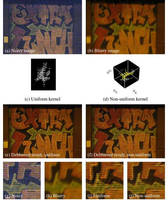
Fig. 13 Deblurring real camera shake blur using a noisy / blurry image pair. A noisy image (a) and blurry image (b) captured with a hand-held camera, shown with the estimated kernels (c–d) and deblurred images (e–f) for the uniform and non-uniform blur models. Note in the close-up that the result using our model (j) has sharper edges and fewer artifacts than that using the uniform model (i). The non-uniform kernel in (d) covers \pm 3^\circ along each dimension
