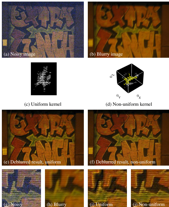
Fig. 13 Deblurring real camera shake blur using a noisy / blurry image pair. A noisy image (a) and blurry image (b) captured with a hand-held camera, shown with the estimated kernels (c–d) and deblurred images (e–f) for the uniform and non-uniform blur models. Note in the close-up that the result using our model (j) has sharper edges and fewer artifacts than that using the uniform model (i). The non-uniform kernel in (d) covers \pm 3^\circ along each dimension
