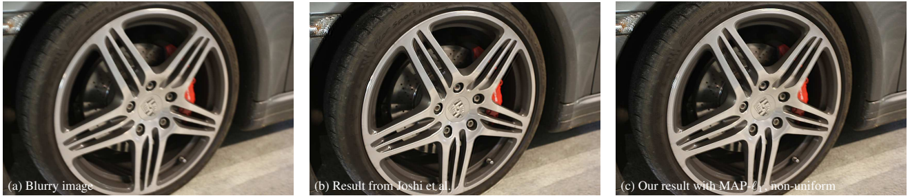
Fig. 11 Blind deblurring of an image from (Joshi et al. 2010). A hand-held image with camera shake (a), from (Joshi et al. 2010), with the deblurred results from the original work (b) and using the MAP- \ell_1 method with our blur model (c). We obtain a comparable result, without the use of additional hardware and without considering the camera’s translation during the exposure, despite the scene being close to the camera.
