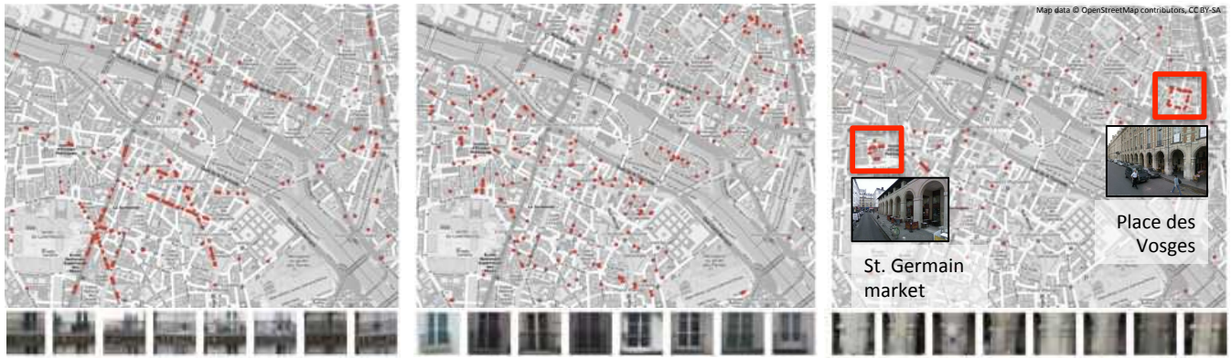
Figure 7: Examples of geographic patterns in Paris (shown as red dots on the maps) for three discovered visual elements (shown below each map). Balconies with cast-iron railings are concentrated on the main boulevards (left). Windows with railings mostly occur on smaller streets (middle). Arch supporting columns are concentrated on Place des Vosges and the St. Germain market (right).
