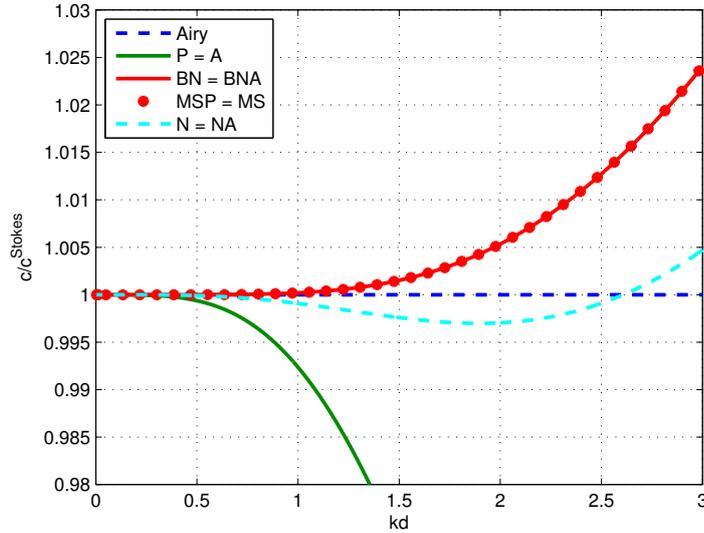
Figure 2: Phase velocity ratio for all the models : P stands for Peregrine (eq. (3)), A for Abbott (eq. (8)), BN and BNA for Beji-Nadaoka and Beji-Nadaoka-Abbott (eq.s (11) and (12) resp.), MS and MSP for Madsen-Sørensen and Madsen-Sørensen-Peregrine (eq.s (14) and (17) resp.), and N and NA for Nwogu and Nwogu-Abbott (eq.s (22) and (26) resp.).
