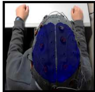
Figure 5: Rear-view window: a virtual brain is superimposed with the back of the user's head. It follows the orientation of the real user's head and enables the perception of what happens at the back of the head (brain).
