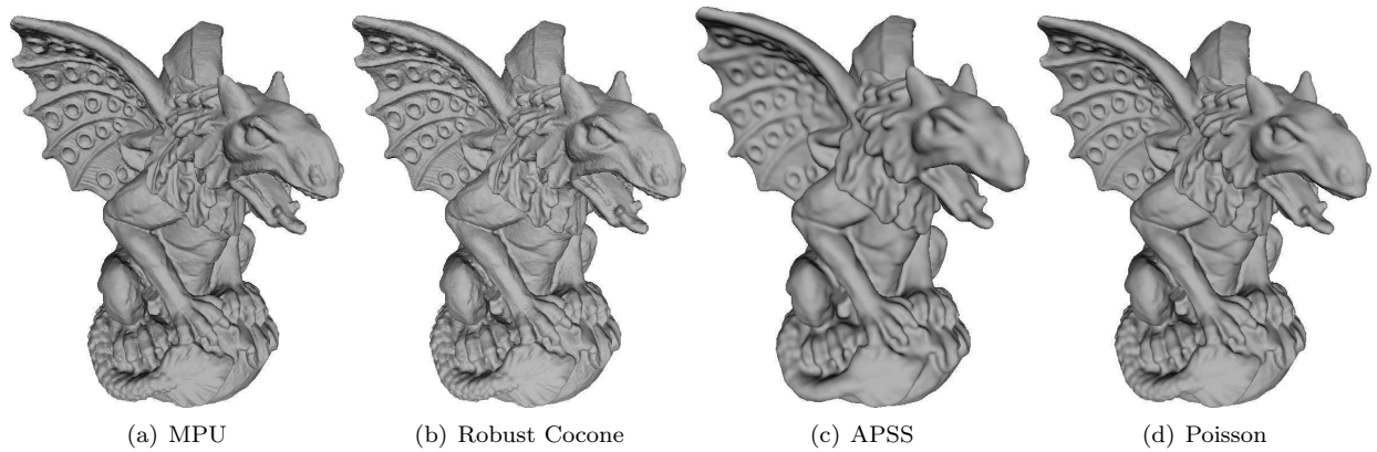
Figure 11: Results of some of the state-of-the-art surface reconstruction methods applied to the Gargoyle dataset. From left to right, the methods tested are MPU (Ohtake et al., 2003), Robust Cocone (Dey and Goswami, 2006), APSS (Guennebaud and Gross, 2007) and Poisson (Kazhdan et al., 2006). With the exception of Robust Cocone, the methods tested require per-point normals, in this case available from the original range scan data. Note that this reference shape poses no problem to any of the methods, and that the results obtained are comparable to those provided by our method, shown in Figure 10 (d).
