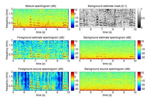
**Fig. 6** Noise/speech separation using REPET-SIM. The mixture is a female speaker (foreground) speaking in a town square (background). The square has repeating noisy elements (passers-by and cars) that happen intermittently. The spectrograms and the mask are shown for 5 seconds and up to 2 kHz. The file is  $dev\_Sq1\_Co\_B$  from the task of two-channel mixtures of speech and real-world background noise of the Signal Separation Evaluation Campaign (SiSEC)<sup>8</sup>.
