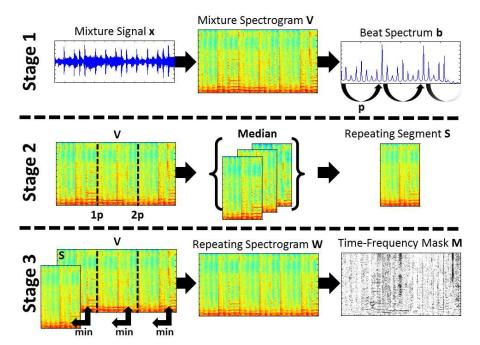
Fig. 1 Overview of the original REPET. Stage 1: calculation of the beat spectrum b and estimation of a repeating period p. Stage 2: segmentation of the mixture spectrogram V and calculation of the repeating segment model S. Stage 3: calculation of the repeating spectrogram model W and derivation of the soft time-frequency mask M.
