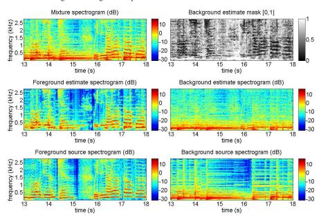
**Fig. 4** Music/voice separation using the adaptive REPET. The mixture is a male singer (foreground) singing over a guitar and drums accompaniment (background). The guitar has a repeating chord progression that changes around 15 seconds. The spectrograms and the mask are shown for 5 seconds and up to 2.5 kHz. The file is *Another Dreamer - The Ones We Love* from the task of professionally produced music recordings of the Signal Separation Evaluation Campaign (SiSEC)<sup>6</sup>.
