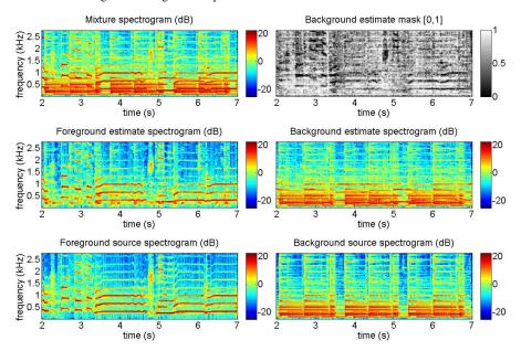
**Fig. 2** Music/voice separation using the original REPET. The mixture is a female singer (foreground) singing over a guitar accompaniment (background). The guitar has a repeating chord progression that is stable along the song. The spectrograms and the mask are shown for 5 seconds and up to 2.5 kHz. The file is *Tamy - Que Pena Tanto Faz* from the task of professionally produced music recordings of the Signal Separation Evaluation Campaign (SiSEC)<sup>3</sup>.
