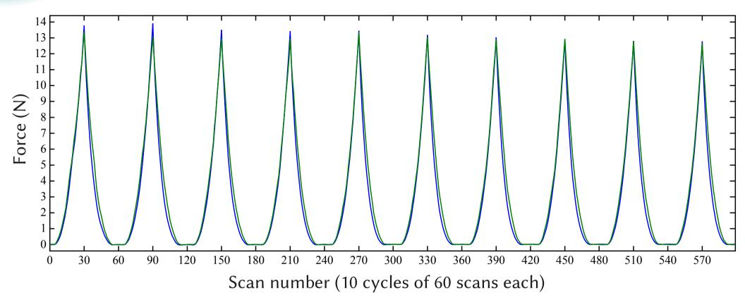
Blue = force measured on the top plate sensor Green = force inferred from the images + measure of E≈23 kPa
