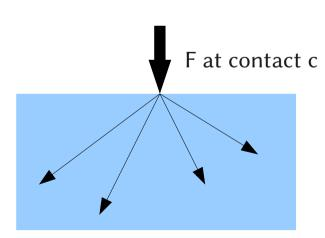
Displacement  $\delta$  induced by F at distance d in the continuous elastic medium  $_{15/17}$
