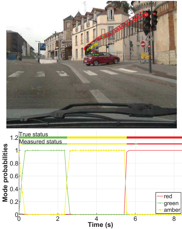
Fig. 9: Result of the algorithm on real data top: Track history plotted on the last frame bottom: Model probabilities for each status through the time
