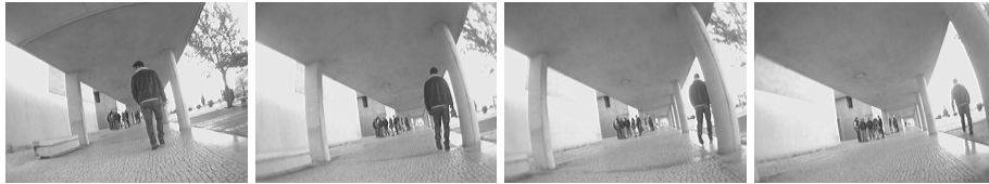
Fig. 6. Bad leader: the person notices the robot and moves aside, giving room for the robot to pass.
