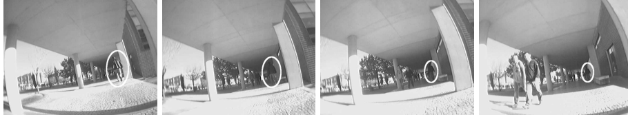
Fig. 7. Bad leader: the subject marked with a white circle moves too fast compared to the robot's speed and gets too far from it.
