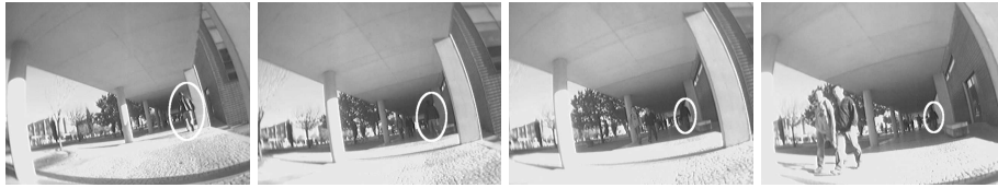
Fig. 7. Bad leader: the subject marked with a white circle moves too fast compared to the robot's speed and gets too far from it.
