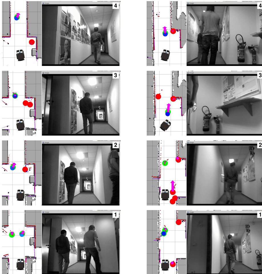
Fig. 15. Two tests on leader switching. On the left column the leader stops and the robot switches to follow another person. On the right a better leader appears on the scene.
