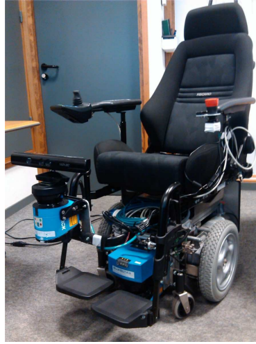
Fig. 10. Experimental platform, showing the two LIDARs and a RGBD camera.
