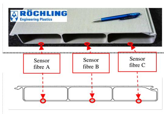
Figure 5: Pultruded profile of a test bridge to demonstrate the sensitive composite box girder.
