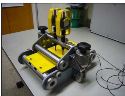
Figure 3: Portable 4-point bending test facility for strain calibration on-site (designed by H. Kohlhoff, BAM).
