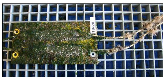
Figure 2: Detailed view at one of the exposed sensor-equipped plates. Clearly can be seen the marine biology vegetation (algae, barnacles and polyps at the leading cable).
