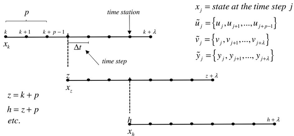
Fig.1 Schematic illustration of sequential deconvolution with notation.
