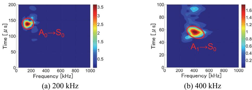
Figure 9: CWT results of A mode transmitting and S mode receiving in the delaminated area
