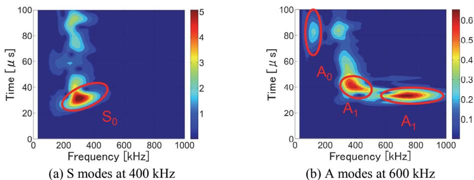
Figure 5: CWT results of same mode transmitting and receiving
