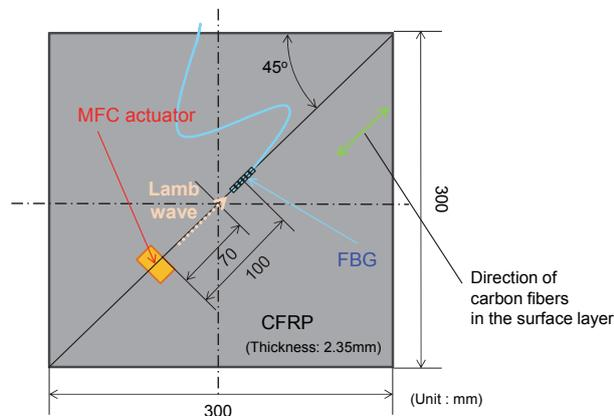
Figure 4: Schematic of the experiment setup for mode separation
