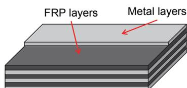
Figure 1: Schematic of FML
