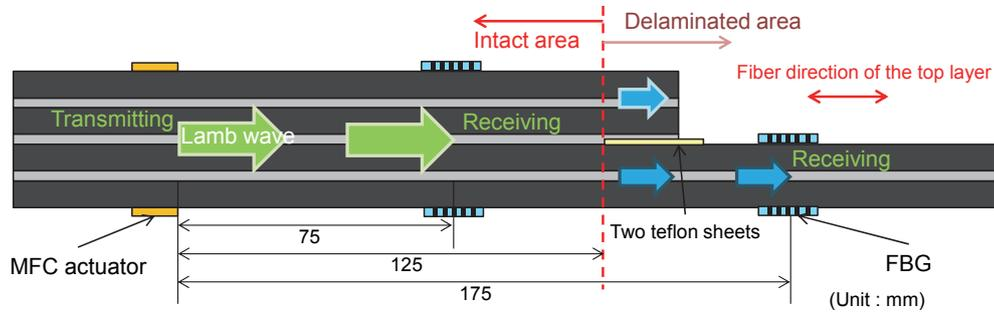
Figure 7: Schematic of the specimen for observation of mode conversions at the delamination tip
