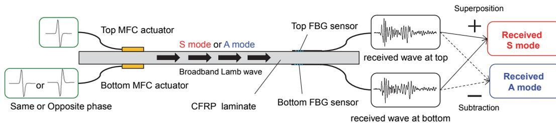
Figure 3: Separation of S modes and A modes by using two MFCs and two FBGs
