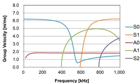
Figure 2: Theoretical dispersion curves of group velocities for the specimen used in this research
