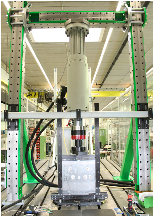
(a) Test bench for the post buckling experiment in our structural laboratory
