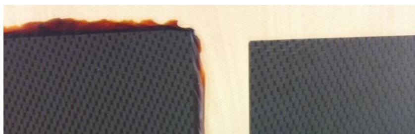
Figure 4: CFRP plates with unfinished resin edges (left) and straight edges (right)
