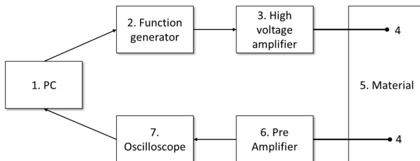
Figure 3: Test Equipment
