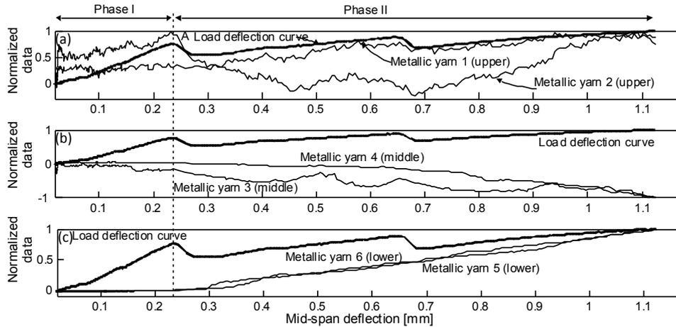
Figure 6: Normalized electrical readings of the metallic yarns in beam M2 and normalized applied load versus mid-span deflection: (a) upper metallic yarns; (b) middle metallic yarns; (c) lower metallic yarns.
