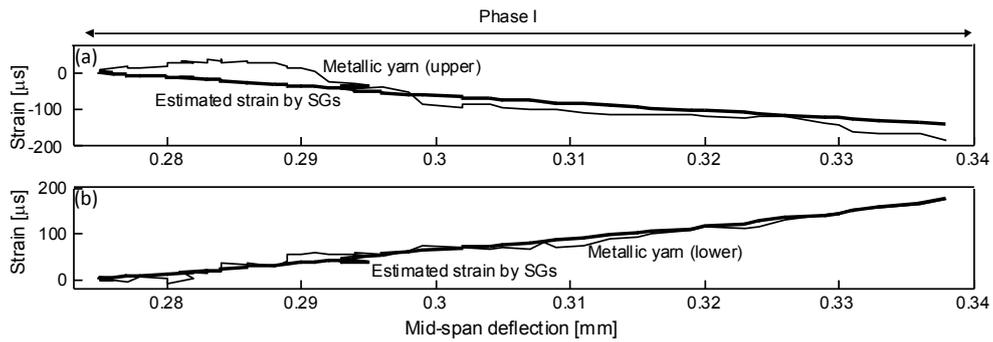
Figure 9: Strain reading of the metallic yarns in beam M1 compared with strains interpolated using the readings of the strain gauges (calibration factor=25  $\epsilon/\mu V$ ): (a) upper yarns; (b) lower yarns.
