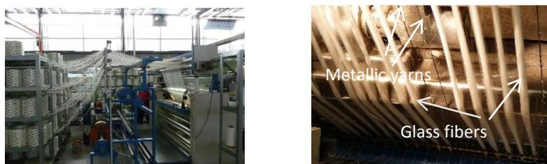
Figure1: Conductive thread insertion into warp knit.
