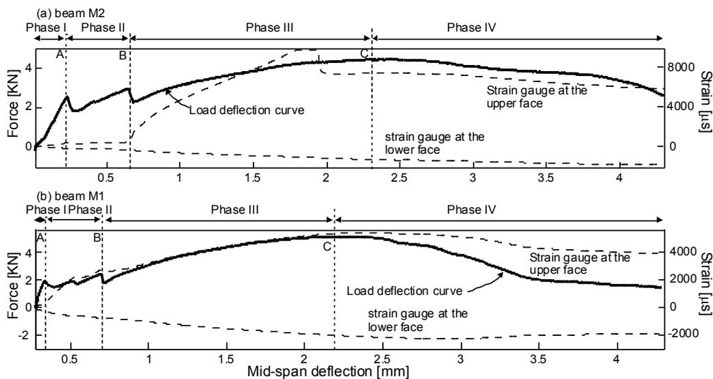
Figure 4: Load-deflection curves and readings of the strain gauges: (a) beam M2, (b) beam M1.
