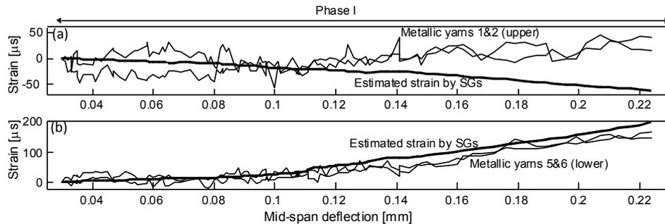
Figure 8: Strain reading of the metallic yarns in beam M2 compared with strains interpolated using the readings of the strain gauges (calibration factor= $45 \text{ } \epsilon/\mu\text{V}$ ): (a) upper yarns; (b) lower yarns.
