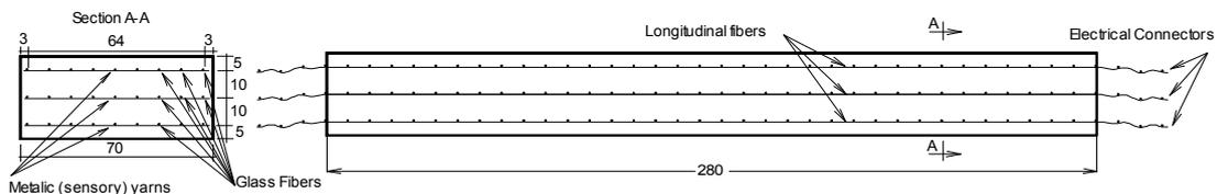
Figure 2: Drawing of the beam.
