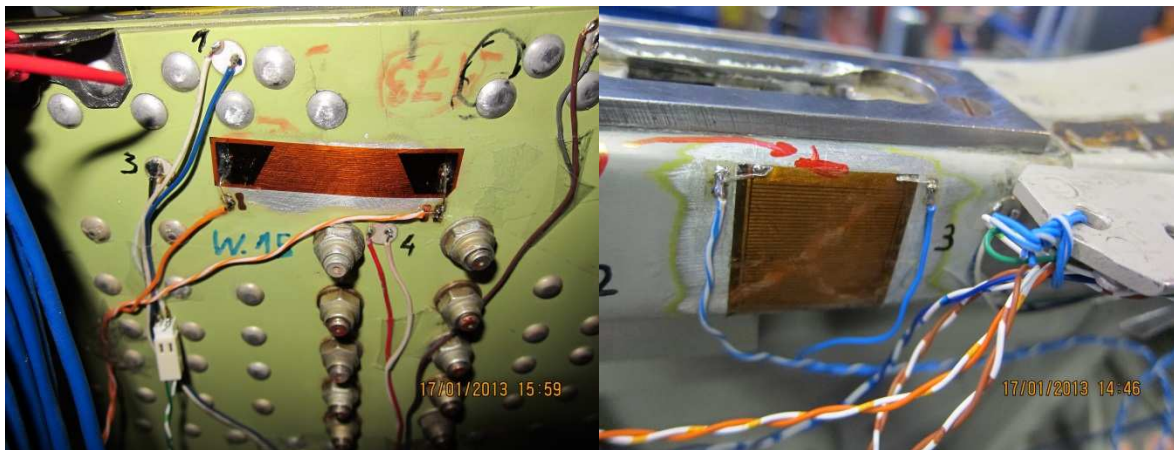
Figure 5. The view of measurement nodes for Resistive Ladders Sensor W.15 (left) and W.19 (right)
