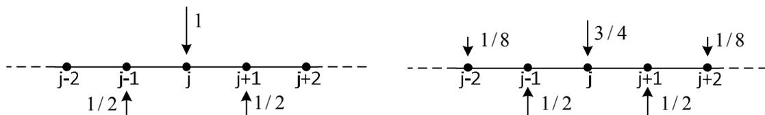
Fig. 5: A load configuration of a hyper-static beam structure that causes concentrated virtual stresses within the region between node  $j-1$  to node  $j+1$  (left figure) and that causes non-zero virtual stresses only within the region between node  $j-2$  to node  $j+2$  (right figure).
