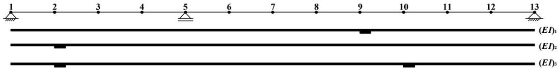
Figure 3. Measurement points and locations of stiffener of the three “damaged” cases of the continuous beam specimen.
