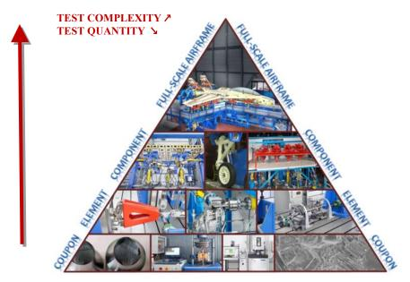
Figure 3: IABG's test pyramid for aeronautic structures
