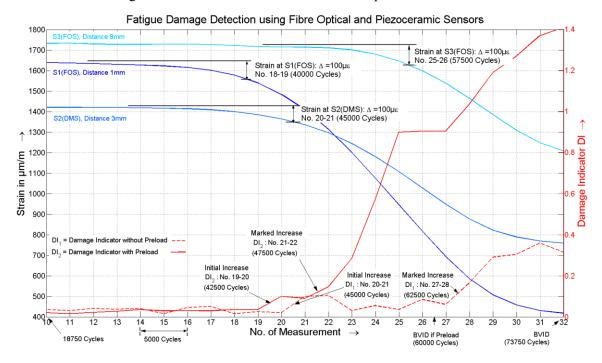
Figure 6: Fatigue Damage Detection starting from the Proportional Limit Stress
