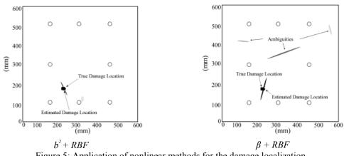
Figure 5: Application of nonlinear methods for the damage localization.
